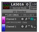
Indicates "rising edge trigger". Indicates "high level trigger".
