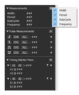
After some items have been selected, move the mouse inside the waveform window, the measurement results of where the mouse stays would display in the measurement window.
